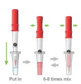
Mix collected sample with an extraction buffer until a latex tablet dissolves perfectly.
