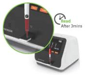
Apply the sample mixture into the sample well of the test device.
