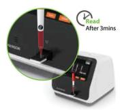
Apply the sample mixture into the sample well of the test device.
